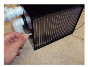
Each LED fixture has 7 LEDs connected in a series string. To connect the LED fixtures to the driver, the fixtures must be connected together so that a single series string of 14 LEDs is formed. This allows both fixtures to operate off of a single Meanwell LPC-35-700 driver.
