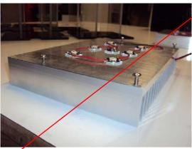
Here is an example of how far the screws should be backed out
